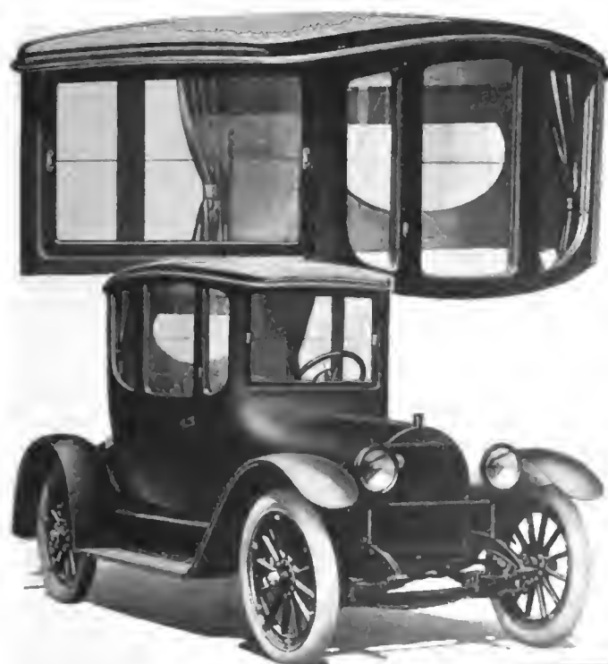
Convertible roadster coupé which gives a luxurious town body for winter or city use and an open roadster for summer work when it is desired to tour without a top. The summer top and windshield are fitted to this body when the coupé is removed
